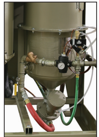
Flange-mounted blast machine on Pulsar® VIP
